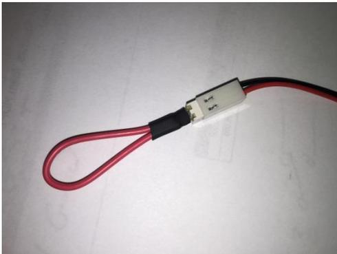
5. Once the remote transmitter has been learned by the opener, you will hear a series of clicks from the motor unit and the lights in the opener (if installed) will flash indicating successful learning of the remote. You can now unplug the program jumper.
